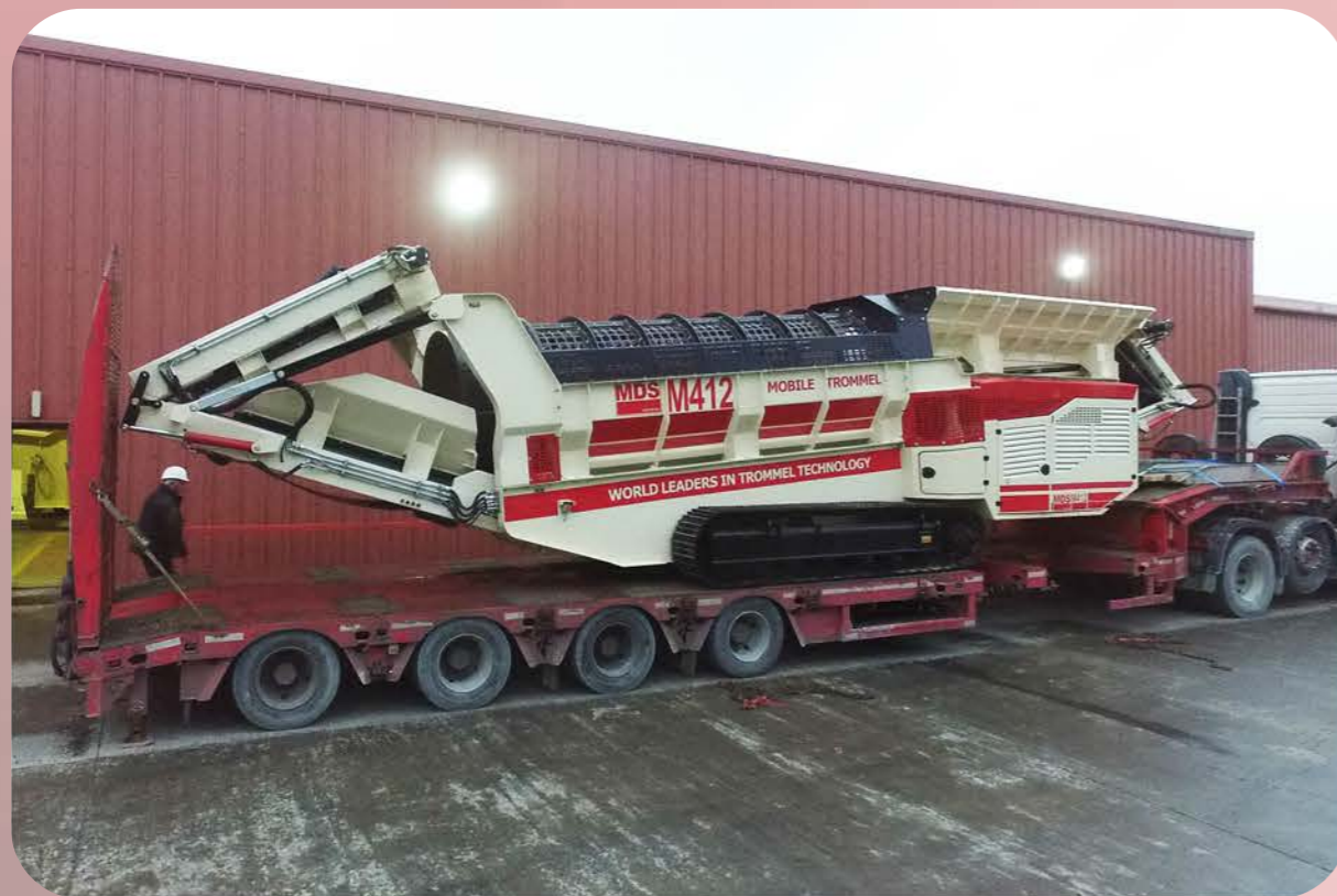
M412 ready to be transported from site to site on a regular trailer
