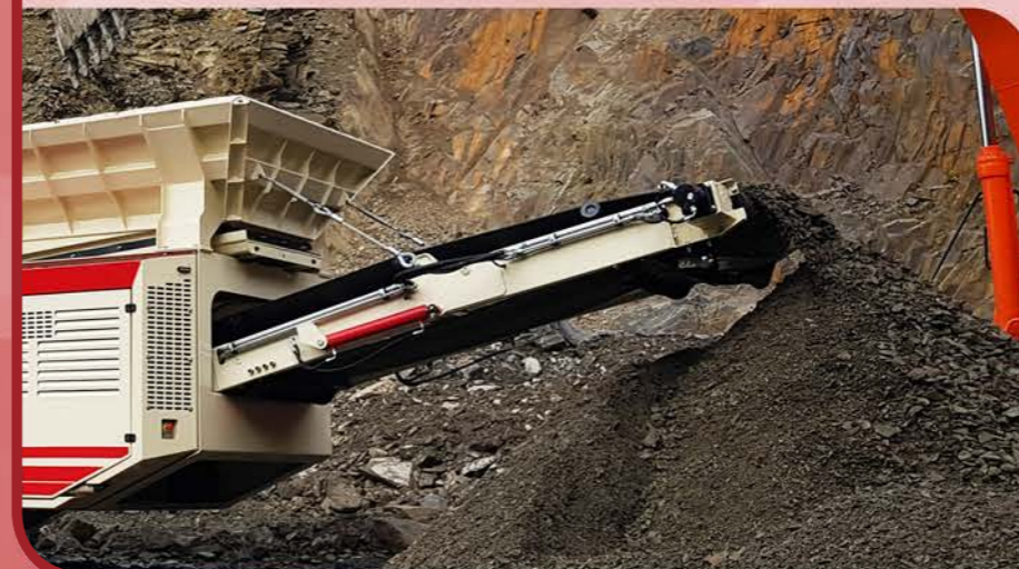
65% Fines through the fines conveyor
